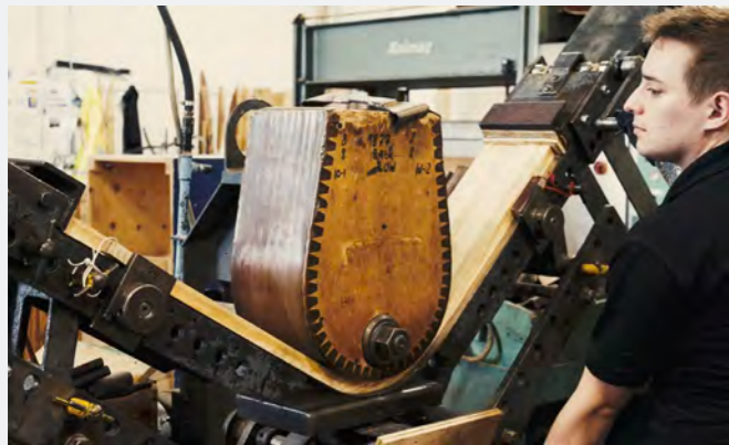
Combining modern CNC machining with traditional steam bending and hand finishing is what makes the 1877 Windsor chair unique.
